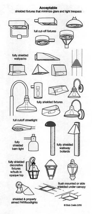
Figure 3: Examples of acceptable fixtures
