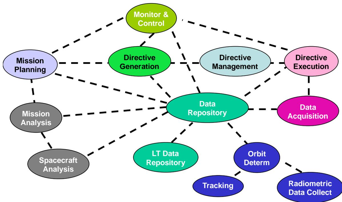
**Figure 5-2: Example of Functional View (Functional Objects and Interactions)**
