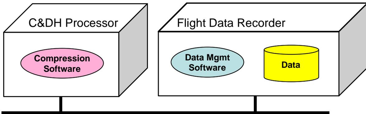
Figure 6-6(b): Connectivity View of Software Compression Approach
