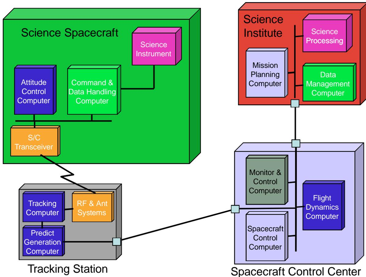
**Figure 6-4: Example of Connectivity View (Node Decomposition)**
